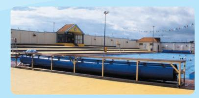
This Reel System provides a solid, hardwearing and attractive surround for your cover and is available in sizes up to 10.4m (34') in length. The majority of Reel Systems up to 9.1m (30') are produced with a 127mm (5") diameter aluminium tube. Reel Systems over this size are produced with a 152mm (6") or a 304mm (12") diameter stainless steel tube. A 6:1 reduction gearbox is fitted as standard for ease of use, alternatively, this system can be motorised.
