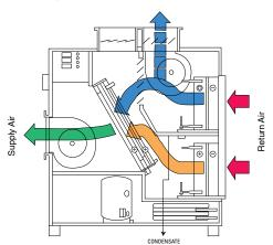
Air temperature set back is a standard feature on each Delta and is controlled by the units time clock. Pool hall temperature is lowered during a chosen set back period for maximum economy. Dampers are automatically adjusted to balance air flows. Unoccupied set back / air heating can be linked to opening / closing of a pool cover.
