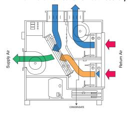
Delta system shown operating on maximum dehumidification. Dampers fully open. Full heat recovery to pool water and hall air.
