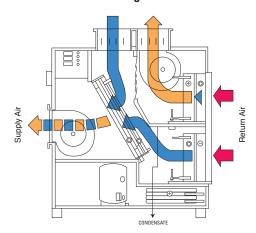
Air conditioning mode. Delta 4 and above all incorporate a true air conditioning facility as standard. This comes into operation automatically whenever the air temperature rises beyond the set point. Surplus warm air is then discharged via the exhaust duct whilst cooler air is introduced to the pool hall.
