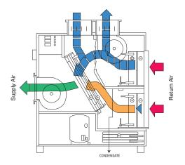
Delta 1/2 operating on light dehumidification with full heat recovery and reduced fresh air stream. LPHW heat available when required.
